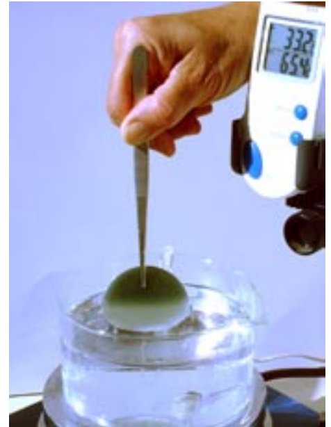
Figure 1 Thermochromic thermosetting plastic possessing a reversible switching between green and colorless.
