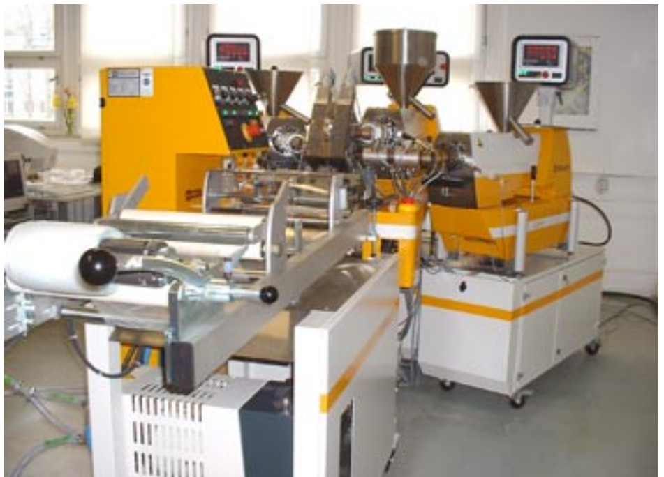
Figure 3 Thermochromic polymer foils with reversible or irreversible switching can be manufactured by extrusion technology.
