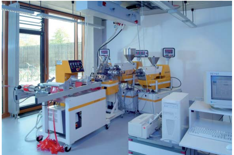
Figure 1 Extrusion equipment for the manufacturing of one and multi layer polymer foils.
